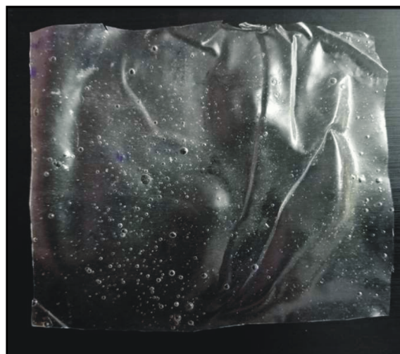
Final Film using 150 ml starch suspension, 6ml glycerol and 6ml garlic extract
